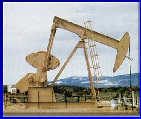
Reverse Mark is a modified conventional unit where the gearbox has been displaced forward so that the angle between the crank arm and the pitman is at 90 degrees when the cranks are level. This results in a faster downstroke than the upstroke.
