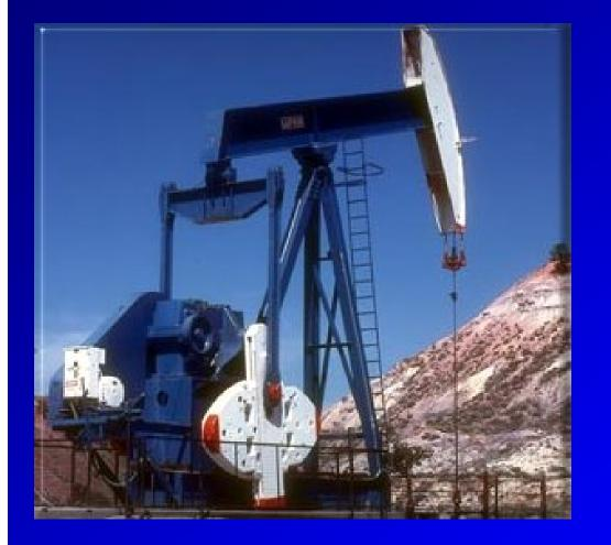
Typically if the unit is stopped and the break released the effect of the counterweights will be greater than the weight of the rods in fluids. As the fluid load is lost due to liquid slippage through the plunger-barrel clearance, the counterweights will come to rest at the 6 o'clock position. The opposite is an indication that the unit is underbalanced (rod heavy).
